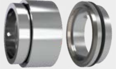
Tungsten - FKM (Viton®) Mekanik Salmatra TuC/TuC/FKM (-50 ... 220 °C)
